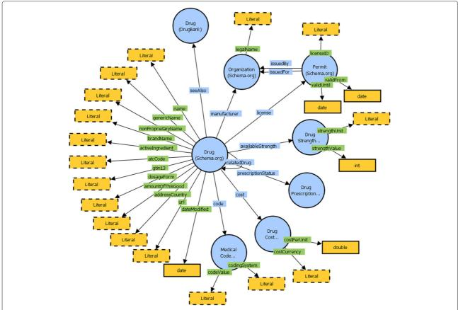
Fig. 2 The RDF vocabulary designed for the drug data domain, comprised of Schema.org classes and properties. For dataset interoperability, it also uses the classes from the ATC Classification Ontology and properties from the DrugBank Ontology and RDFS
